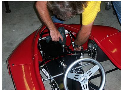
Once you are sure that you are sure that you are sure.., go ahead and drill a 1/4 inch hole in the 2 bolt holes towards the back of the nose.
