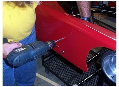
You will see the light shine through the hole in the tab to the outside of the body in the exact spot that you need to drill the hole. Make sure that the body is firmly up against the tab and that the flashlight is not at an angle to the tab because this will make the light shine off center to where the hole needs to be.
