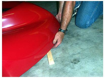
When you think you have it close, place a 1 x 2 or something of similar size underneath the nose at a point just below where you will be drilling the holes through the floor pan.
