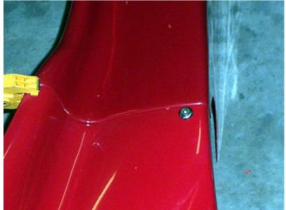
When you get done, the top of the bolt and the conical washer should look like the picture on the left. The bolt head should be flush with the top of the conical washer. This is not as important as the side panel bolts but it looks really nice and clean.
